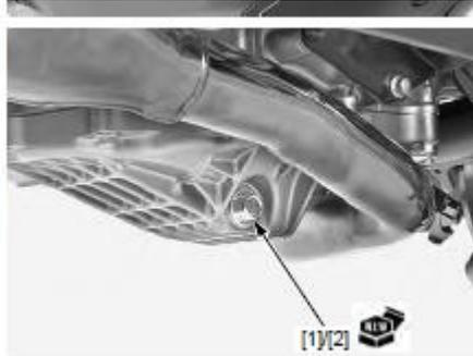
Apply engine oil to a new oil filter cartridge threads and O-ring.
