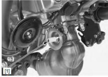
Remove the wire grommet [1] from the right crankcase cover.
